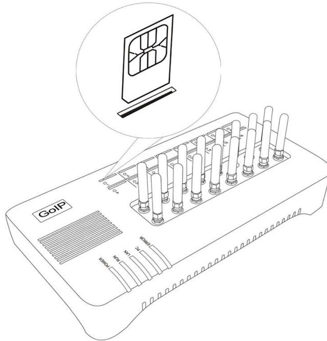
For GoIP-32, the SIM card insertion orientation is shown in the figure below. The cut corner is pointing downward with the metal contacts facing the front of the GoIP.
