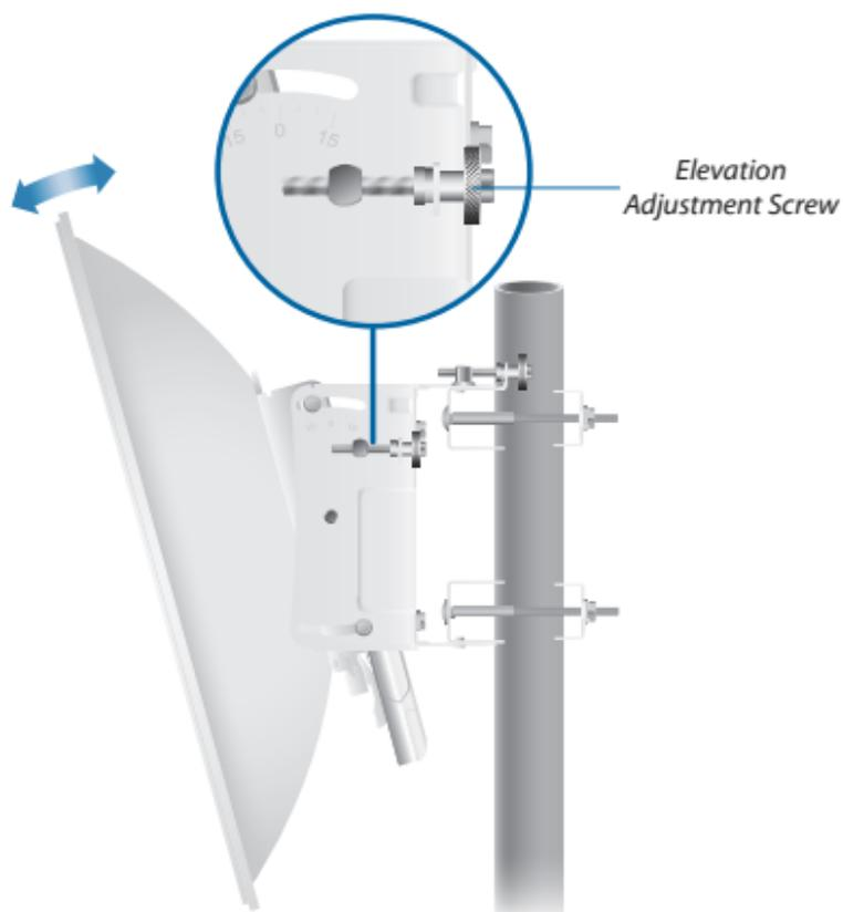
10. Lock the alignment by tightening the eight hex head bolts to 25 N-m.
