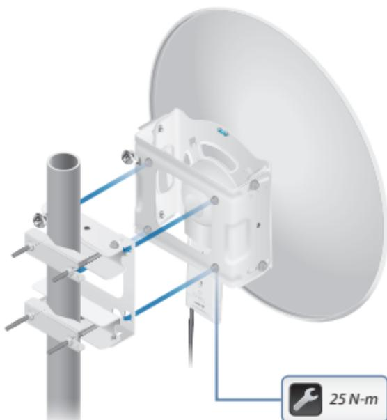
7. Before adjusting the azimuth and elevation angles, ensure that these eight hex head bolts are loose enough to allow movement.
