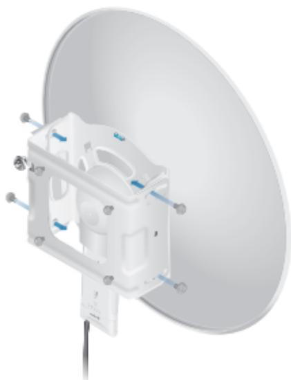
4. Attach two *Pole Clamps* to the *Azimuth Alignment Bracket*.
