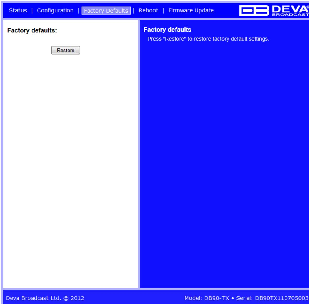
On the above picture is shown the Factory Defaults page. Restoring DB90-TX to its Factory Defaults can be done by following the next steps:
