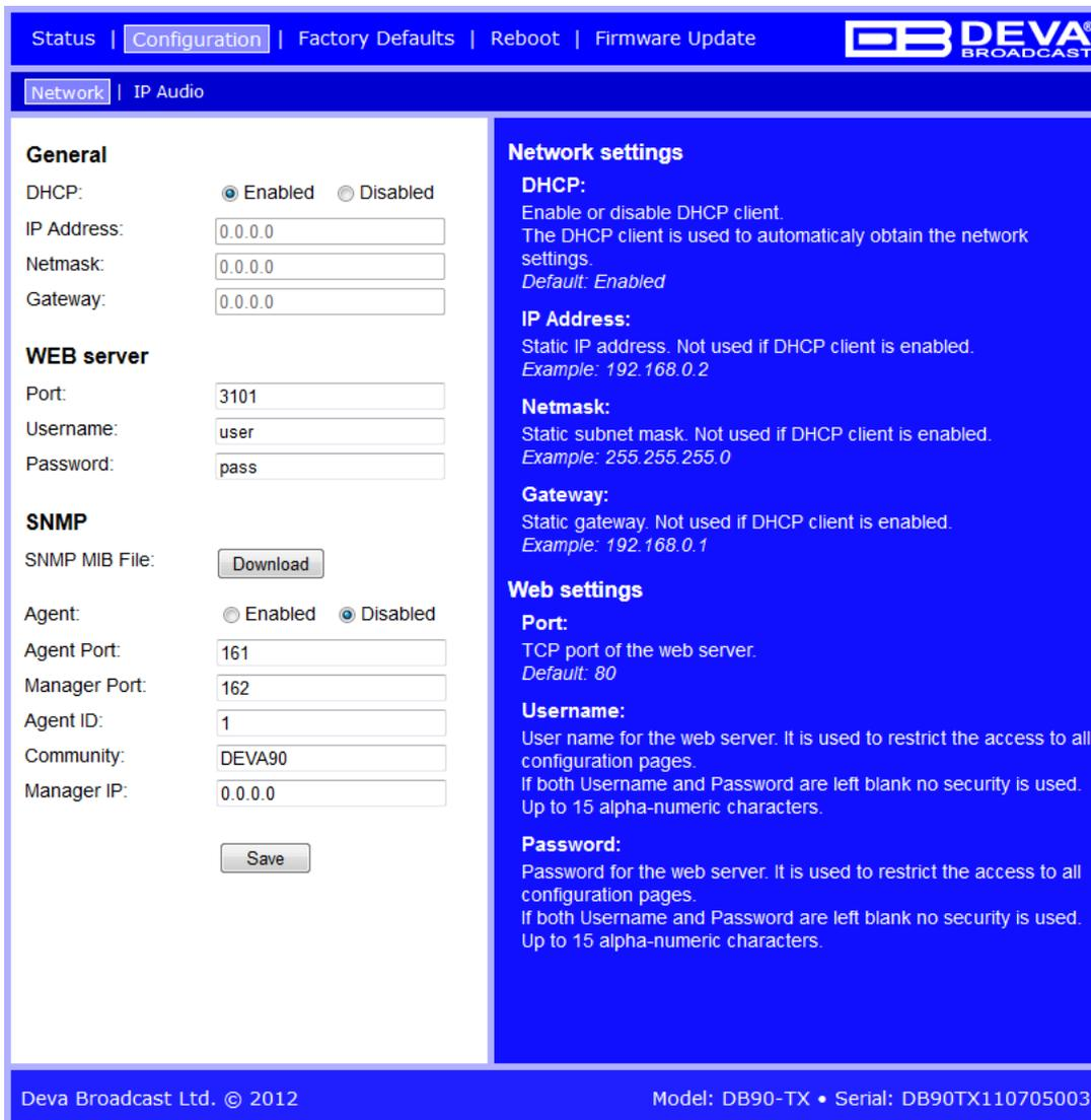
The screenshot shows the configuration page for the DB90-TX device. The top navigation bar includes 'Status', 'Configuration' (selected), 'Factory Defaults', 'Reboot', and 'Firmware Update'. The 'Network' tab is active, with 'IP Audio' as a sub-tab. The interface is divided into two main sections: 'General' and 'Network settings'.
